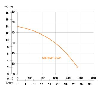
Shaft Speed: 1450 rpm Outlet: 100mm, 4in
